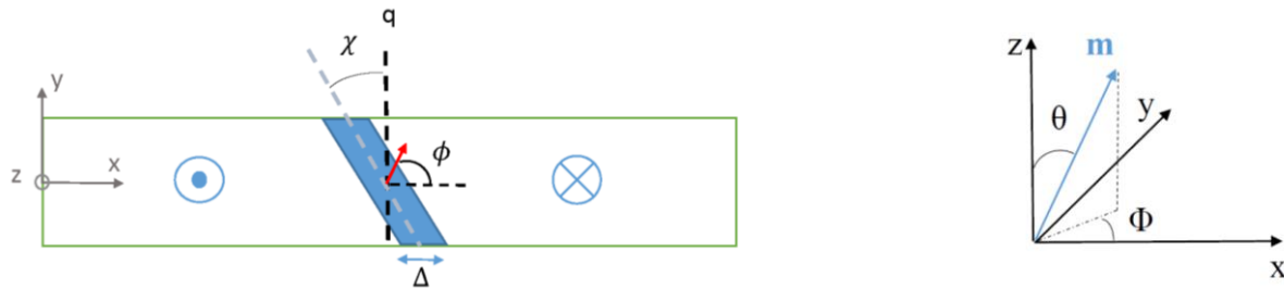
(a) Top view of the nanowire, showing the coordinates q , \Delta and \chi .
