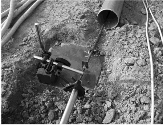
Fig. 8. View of the devices used for the measurement of the anchoring plate displacements.
