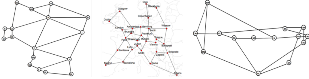
Fig. 1: The considered network topologies 11 . Left) German. Average link length 207 km Middle) Pan-EU. Average link length 637 km Right) US. Average link length 1463 km.
