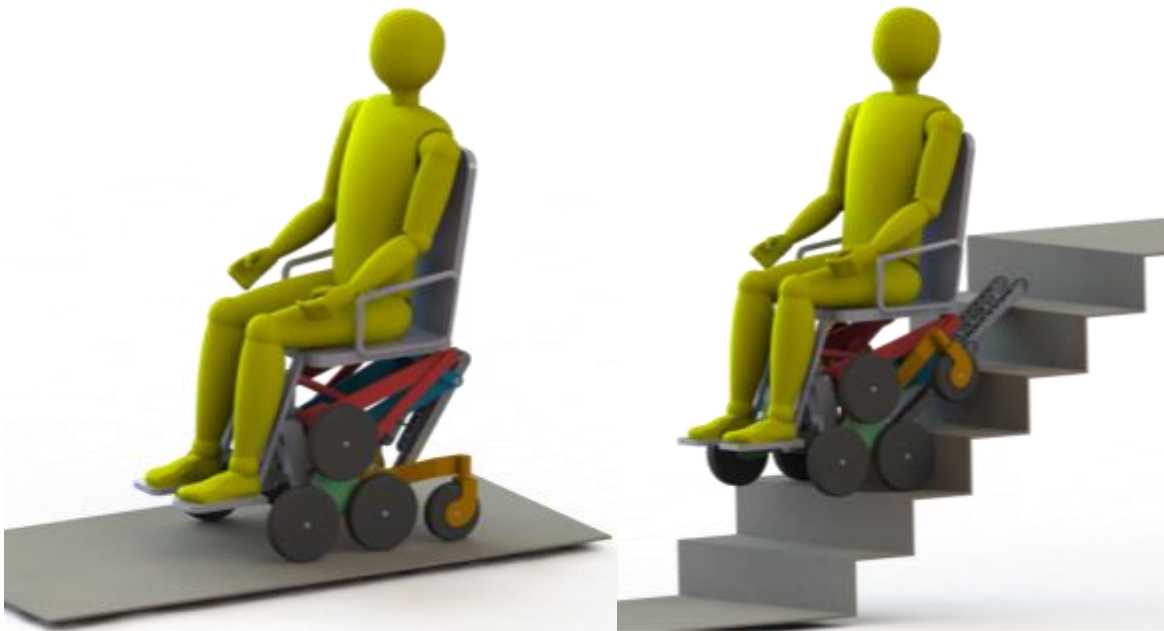
Figure 12 – Constructive representation of the whole wheelchair on flat ground and on stairs
