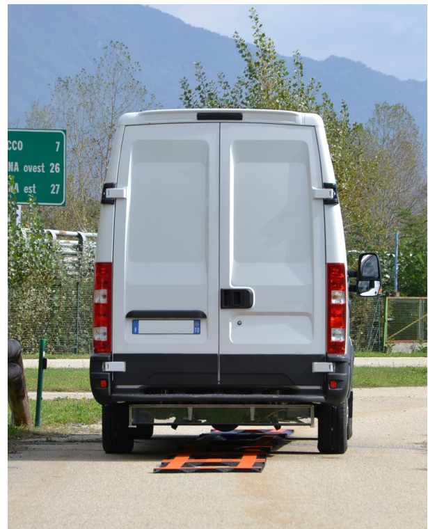
Fig. 12: Back of the vehicle during the CWD operation. Under the vehicle plane is visible the receiving structure mounted.
