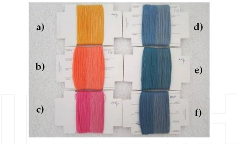
Figure 3. Dyeings with 0.5% selected dyes: (a) Levafix Amber CA, (b) Remazol Orange RR, (c) Remazol Red RB 133%, (d) Remazol Navy GG 133%, (e) Remazol Black B 133%, (f) Remazol Blue RR (for each shade: untreated yarn on the left side, UV faded on the right side).
