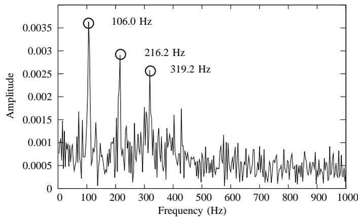
Fig. 9. Envelope spectrum emphasizing the bearing defect
