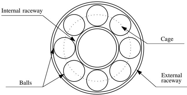
Fig. 2. Sectional view of a bearing model [10].
