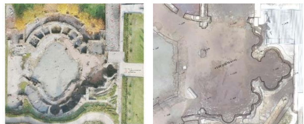
Figure 3: (left) The orthoimage from the UAV acquisition and (right) detail of top view of the vectorialized laser point cloud
