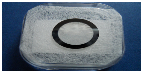
Figure 3. The diamond disk (transparent area) stuck onto the silicon ring (black ring).
