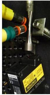
Fig. 2. Typical measuring system configuration in an ultrasonic test.
