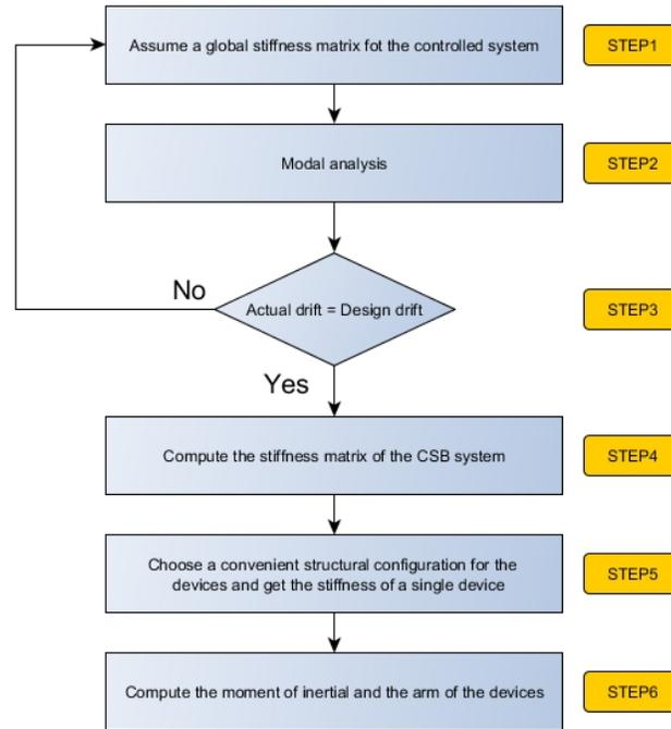
Figure 4- Flowchart of the CSB design scheme
