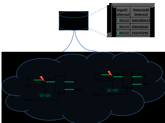
Fig. 6. Logic test intra-cell defect grading
