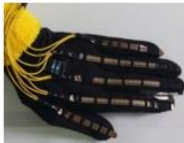
Fig 9 Glove with Flex Sensors
