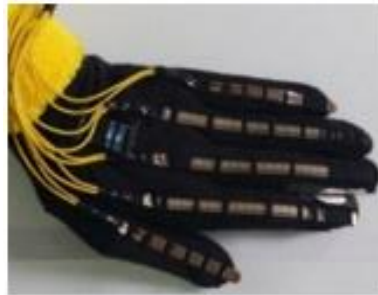
Fig 9 Glove with Flex Sensors
