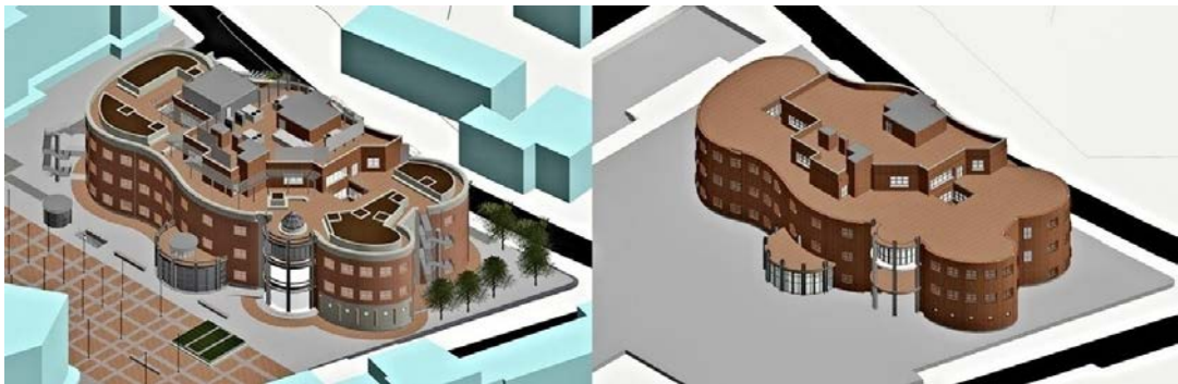
Fig. 1. Comparison between the architectural and the energy model.
