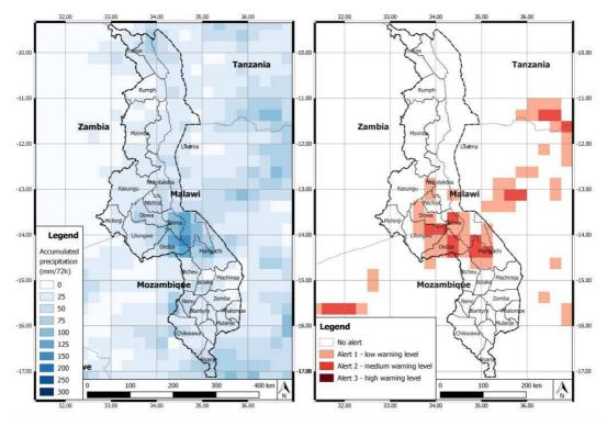
Figure 5.10 72h TRMM-3B42RT accumulated precipitation and Extreme Precipitation Alerts (05-07 January 2013)
