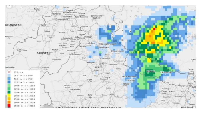
Monitoring from TRMM data: accumulated precipitation over past 24h (www.ithacaweb.org)
