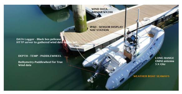
Figure 5.17 Weather boat instruments
