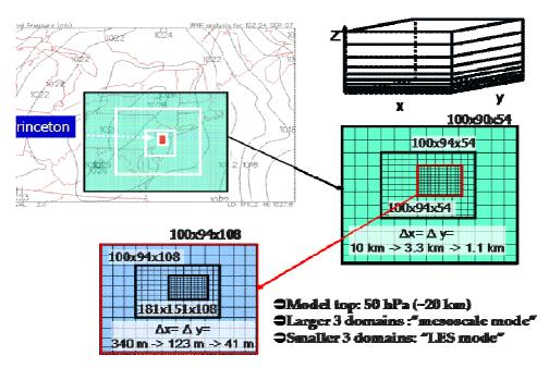
Figure 3.1 Initialization of a mesoscale model with a global model (source http://efm.princeton.edu/)
