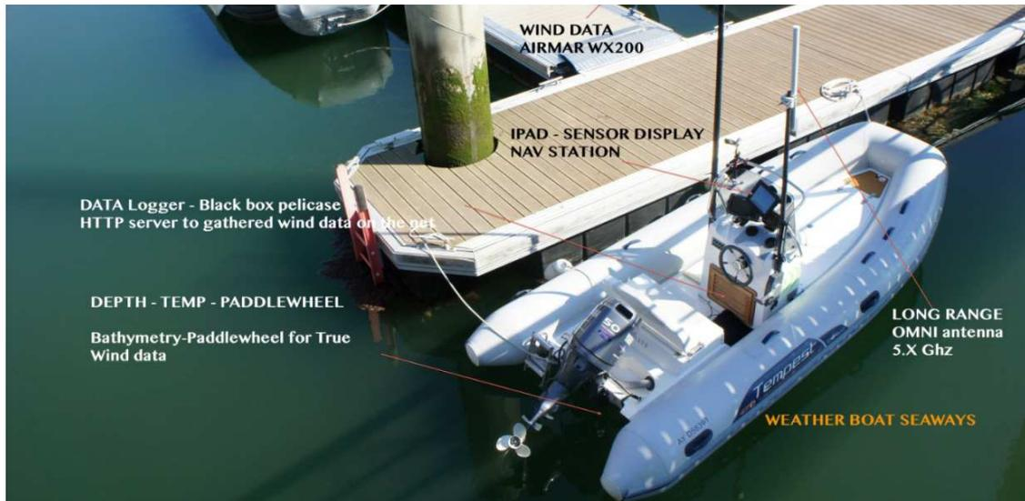
Figure 5.17 Weather boat instruments
