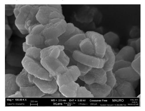
Figure 1.5: FESEM images of MSU-H-F aggregates.
