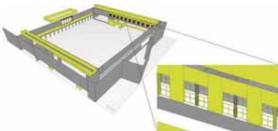
Fig. 9 – Elements exported by gbXML which do not maintain their volumetric characteristic
