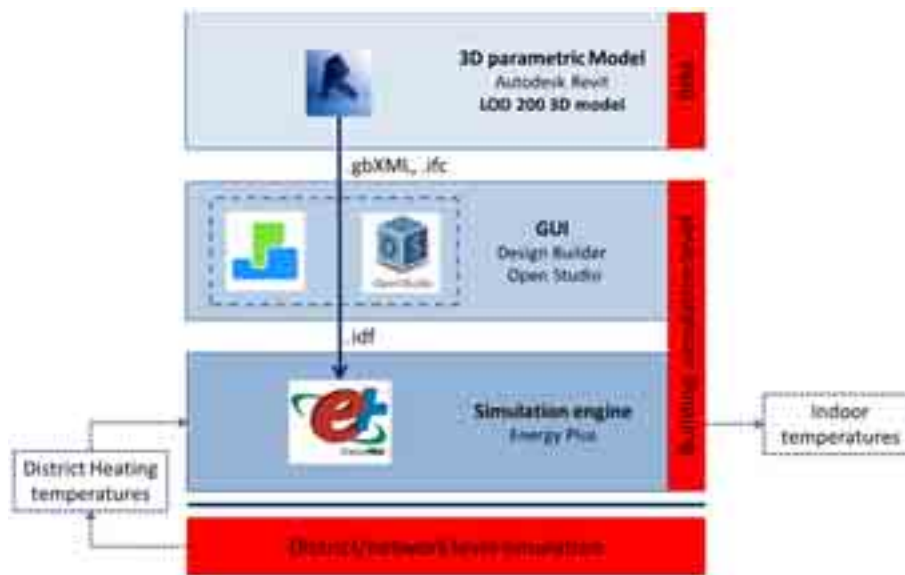
Figure 41 Interoperability process for Building simulation level
