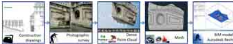
Figure 14 Workflow for the generation of the grand staircase of Valentino Castle
