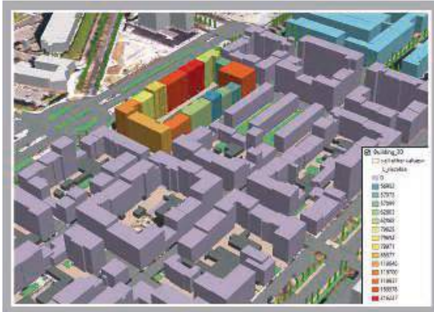
Fig. 14 – The GIS data about the heating consumption of the buildings for a selected block.
