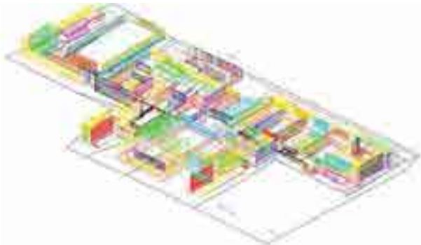
Figure 3. Survey of the Main Campus realized using a total station. (realized by Eraldo Mondino and Daniele Zaccaria)
