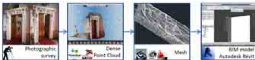
Figure 13 Workflow for the generation of the major port of Valentino Castle
