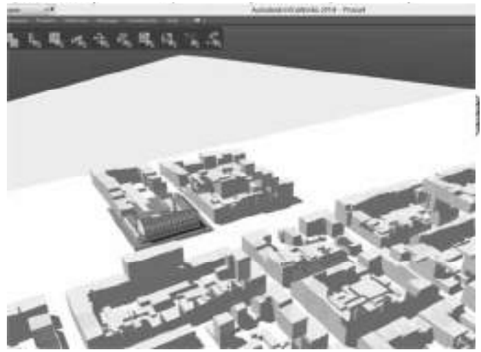
Figure 4. the Coppino model and the Building's shapefile imported on Infracworks. (the model was developed by Paolo Marcia)
