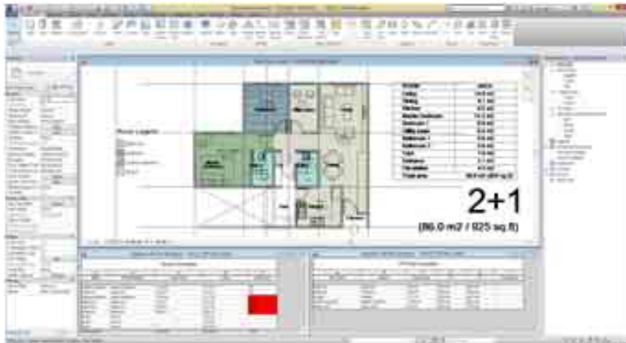
Figure 71 BIM model of a PR1MA unit example with the use of a Key schedule
