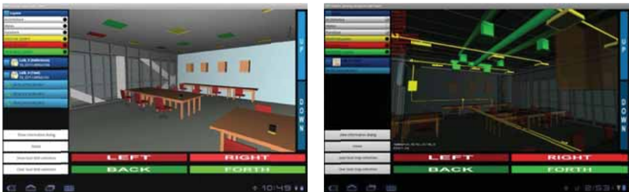
Fig.6: Visualization of the architectural model using a Tablet and of each system using different colours.
