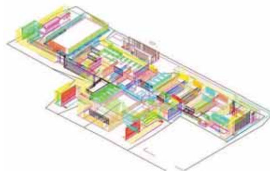
Fig. 1 – Survey of the Main Campus realized through a total station
