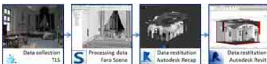
Figure 18 Workflow for the creation of a BIM model of Albergo dei Poveri
