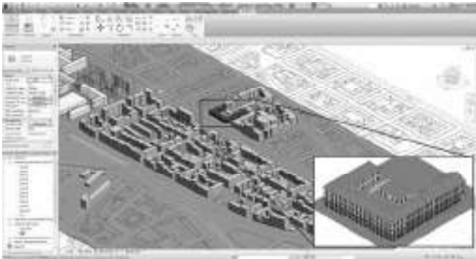
Figure 2. The 3D model of the context and of the Coppino Primary School developed by Pamela Scaramozzi with Revit
