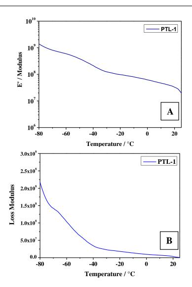
**Figure 3.5** Modulus profile (a) and loss modulus profile (b) of PTL-1 sample, in which the results are shown for DMTA tests carried out between –80 to 30 °C. Above 20 °C, the test failed due to the extra-soft characteristics of the polymer membrane if compared to the applied force from the instrument (10 N).
