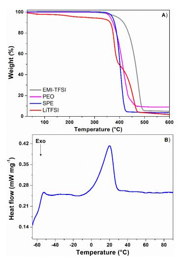
Figure 2.4. Thermal characteristics of the materials: a) TGA profiles and b) DSC traces.
