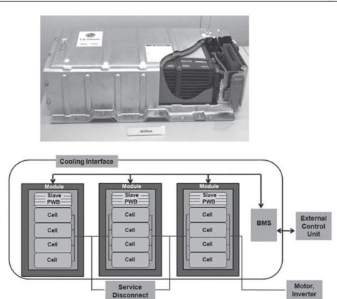
Figure 1.9. A battery pack for HEVs. Reproduced with permission from [2].
