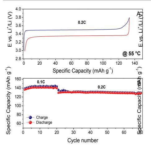
**Figure 2.9**. Cycling behavior of the solid polymer lithium cell assembled by contacting the LiFePO<sub>4</sub>-based electrode/polymer electrolyte with a lithium metal anode in the 3.0 - 3.8 V vs. Li<sup>+</sup>/Li range at different temperatures: a) constant current charge/discharge potential vs. specific capacity profiles extracted from cycle 70 at 0.2C rate and b) specific capacity vs. cycle number plot at different C rates at 55 °C.
