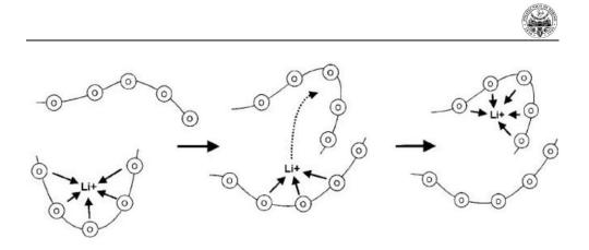
**Figure 1.15** Schematic representation of the coordination site of lithium ions in PEO and its ion conducting mechanism. Reproduced with permission from [62]
