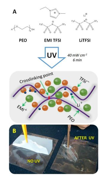
**Figure 2.1 (a)** Sketched representation of the UV process along with the components used in this study and the hypothesized interlinking of PEO polymer chains encompassing imidazolium-based RTIL. **(b)** The real aspect of the polymer electrolyte formed after UV exposure , which is almost transparent, tack free, flexible and easy to manage.
