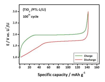
**Figure 3.14** Representative charge/discharge profiles of a cell assembled with the configuration of Li/PTL-1/TiO<sub>2</sub>. The cycling test was performed at 20 °C at a current density of  $0.1 \text{ mA cm}^{-2}$ .
