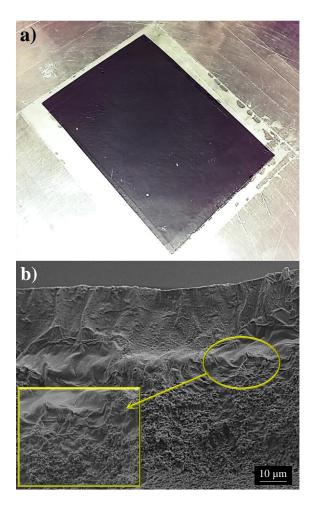
**Figure 2.8.** a) Photograph of a freshly prepared self-supporting multiphase electrode/electrolyte composite obtained by direct hot-pressing and *in situ* photopolymerization of the polymer electrolyte on top of the LiFePO<sub>4</sub> composite electrode; b) Cross-sectional FESEM images illustrating the morphology of the multiphase electrode/electrolyte composite at different degree of magnification.
