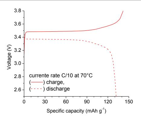
**Figure 4.19** Constant current charge/discharge potential *vs.* specific capacity profile extracted from cycle 2 at C/10 rate.
