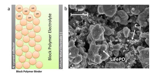
**Figure 4.17** (a) Sketched representation of the cell assembly, where the percolation of the polyelectrolyte in the whole electrode structure is clearly evidenced (b) FESEM image of the composite electrode.
