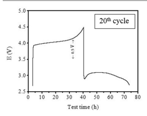
**Figure 3.17** Charge/discharge curve of a lithium test cell assembled with a configuration of Li/PTL-1/LiFePO<sub>4</sub>. The test was performed at 0 °C at current densities of 0.01 mA cm<sup>-2</sup>.
