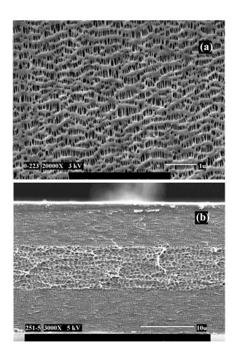
**Figure 1.12** Scanning electron micrographs of Celgard<sup>®</sup> 2325 (PP/PE/PP) separator used in lithium-ion batteries: (a) surface image and (b) cross-section image. Reproduced with permission from [34].
