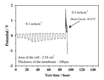
**Figure 3.12.** Galvanostatic cycling curve obtained for Li/PTL-1/Li symmetric cell at fixed current densities of 0.1 mA cm<sup>-2</sup> and 0.3 mA cm<sup>-2</sup> at 25 °C.
