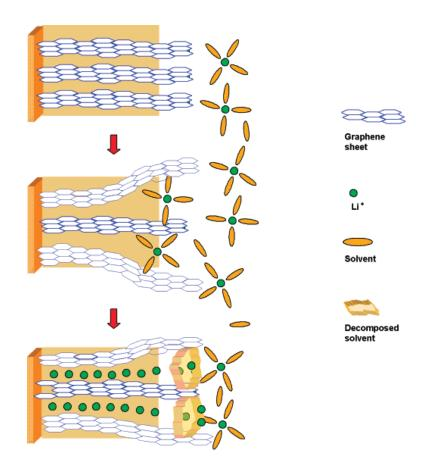
Figure 1.7 Schematic illustration of the SEI formation mechanism. Reproduced with permission from [15].
