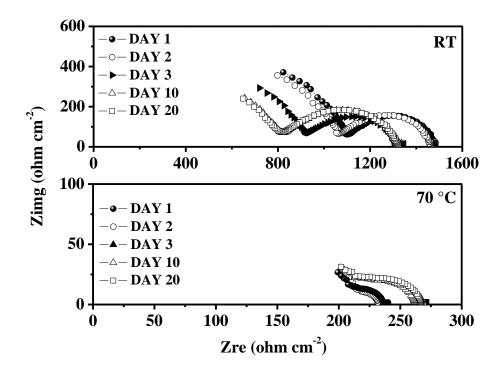
**Figure 5.7** Nyquist plots representing the time evolution of the impedance profile corresponding to the change in interfacial resistance for Li/GPE/Li symmetric cells tested at room temperature (top) and at 70 °C (bottom).
