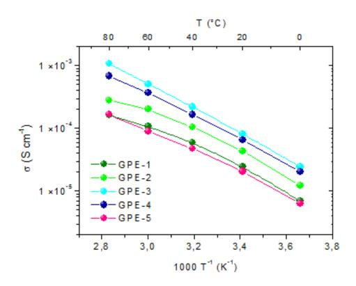
**Figure 5.3** Plot of ionic conductivity against the inverse temperature for the prepared GPEs with different amounts of lithium salt monomer.
