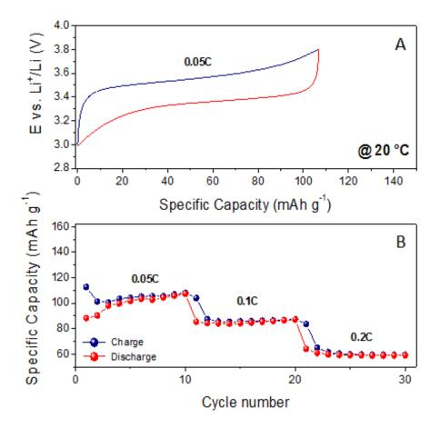
**Figure 2.10**. Cycling behavior of the solid polymer lithium cell assembled by contacting the LiFePO<sub>4</sub>-based electrode/polymer electrolyte with a lithium metal anode in the 3.0 - 3.8 V vs. Li<sup>+</sup>/Li range at different temperatures: a) constant current charge/discharge potential vs. specific capacity profiles extracted from cycle 10 at 0.05C rate and b) specific capacity vs. cycle number plot at different C rates at 20 °C,
