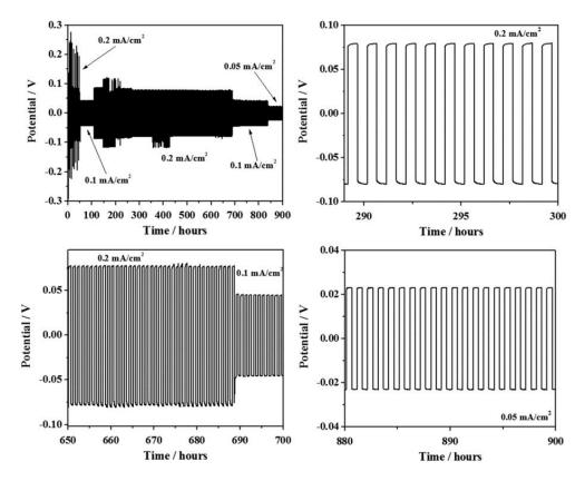
**Figure 3.13.** Potential vs. test time of lithium stripping and plating of a symmetrical lithium cell at various current rates (i.e., 0.05, 0.1, 0.2 mA cm<sup>-2</sup>) at 25 °C.
