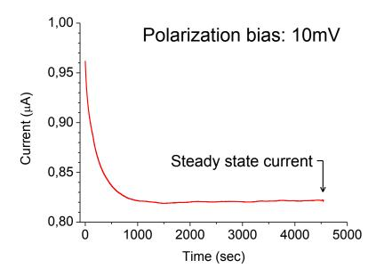
**Figure 4.16** Lithium-ion transport number analysis: (a) Typical Nyquist plot of the a.c. impedance of a Li | LiBC-1 | Li cell at 70 °C, (b) current variation with time during polarization of the symmetrical lithium cell.
