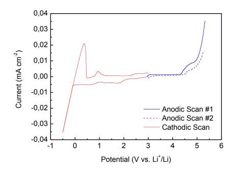
**Figure 4.14**. Electrochemical stability window obtained by CV at 1 mV s<sup>-1</sup> for LIBC-1 at 70 °C.
