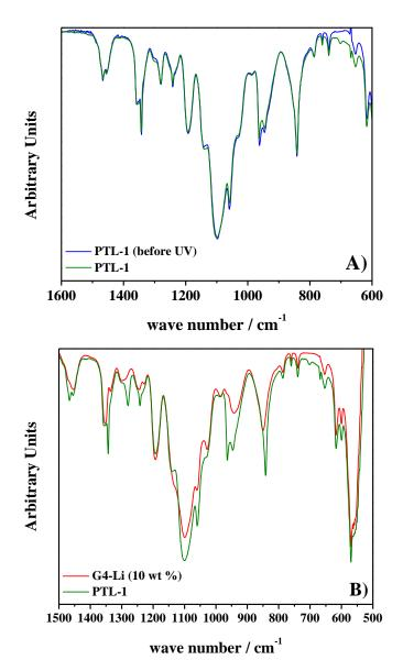
**Figure 3.7** (a) FTIR profiles of PTL-1 before and after UV curing; (b) FTIR profiles of PTL-1 and liquid TEGDME-LiTFSI. The tests were carried out at room temperature.
