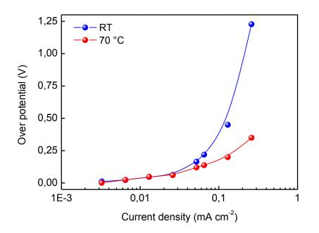
**Figure 5.8.** Plot illustrating the potential as a function of the current rate for a Li/GPE/Li symmetric cell at RT and 70 °C while performing lithium plating/stripping processes at different current densities.
