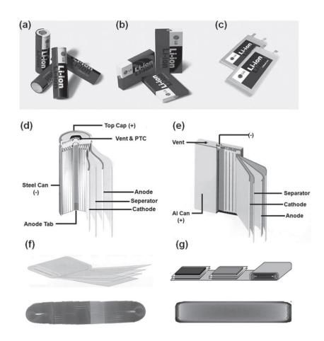
**Figure 1.8** Three different types of commercially available cells of lithium ion batteries: cylindrical (a, d), prismatic (b, e) and polymer (c, f, g) cells. The assembly of cathode, separator and anode is winded (f) or stacked (g) in a pouch of polymer type cells. Reproduced with permission from [2].
