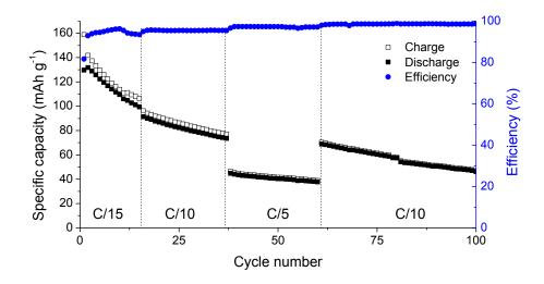
**Figure 4.18** Specific capacity vs. cycle number profile of the Li/LiBC-1/LiFePO<sub>4</sub> cell at different charge/discharge rates at 70 °C.
