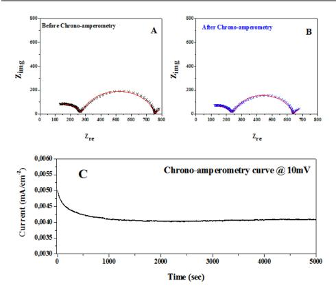
**Figure 3.9. (a,b)** Nyquist plot of a membrane assembled in a symmetric cell (Li/PTL-1/Li) and tested at 20 °C in the frequency range between 2 MHz and 0.1 Hz, before and after the chrono-amperometry test; **(c)** Chrono-amperometry curves obtained for PTL-1 containing cell, tested at 10 mV polarization until obtaining a steady state current under open circuit potential conditions. Tests were carried out for all the samples, but only PTL-1 is showed as the representative.
