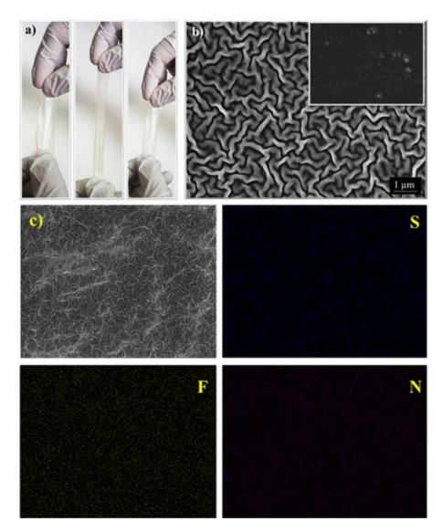
**Figure 2.2** a) Appearance of the light-cured crosslinked polymer electrolyte sample upon manual elongation, b) FESEM analysis at high magnification of the sample surface, c) focus on the area ( $30 \ \mu m \times 30 \ \mu m$ ) of the image where EDX analysis was carried out, along with the following images in which S, F and N indicate the distribution of sulphur, fluorine and nitrogen, respectively, of TFSI<sup>-</sup> anion in the selected area of the sample.
