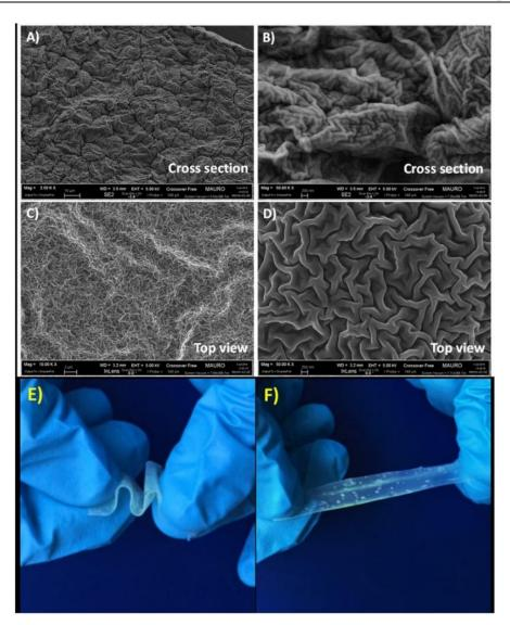
**Figure 3.2.** Micrographs showing the overall morphology of sample PTL-1: cross-section under secondary electron mode (a,b) and top view (c,d), at different magnifications; (e,f) shown the images of the sample PTL-1 (at 25 °C) under stretch and bend mode, demonstrating the mechanical integrity and excellent elasticity.
