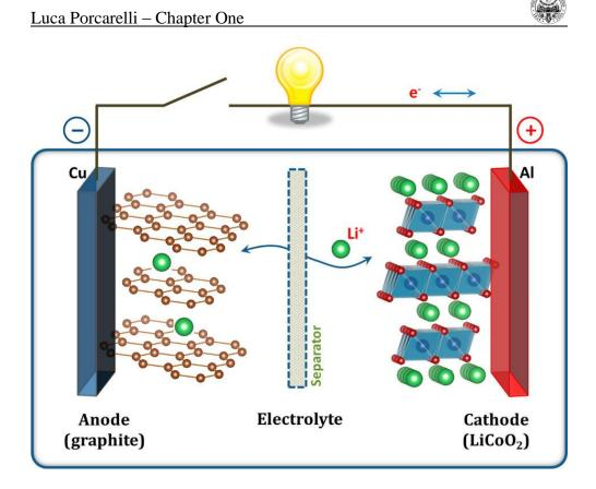
Figure 1.6 Schematic representation of a lithium-ion cell. Reproduced with permission from [4].
