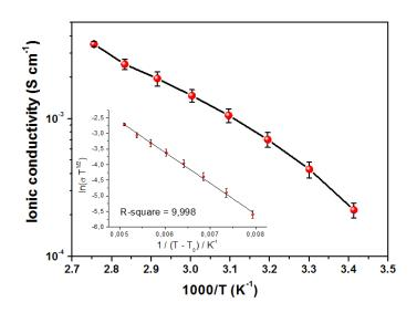
**Figure 2.6.** Arrhenius plot for ionic conductivity as a function of temperature of the polymer electrolyte membrane (in the inset, the fitting by means of the VTF equation). Data obtained by impedance spectroscopy.
