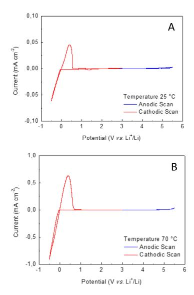
**FIGURE 5.6** Electrochemical window of GPE-3 obtained by CV in the -0.5 - 5.5 V vs. Li<sup>+</sup>/Li interval at a scan rate of 0.2 mv s<sup>-1</sup> and different temperatures: (a) 25 and (b) 70 °C.
