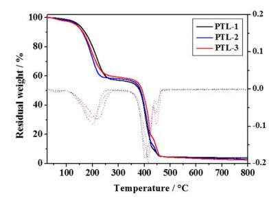
**Figure 3.4** Thermogravimetric analysis (TGA) of the same series of ISPEs along with related differential curves (dotted lines of same colour code). Taking into account the experimental errors related to the measurement and the sample preparation, all weight losses are consistent with the polymer electrolyte compositions.
