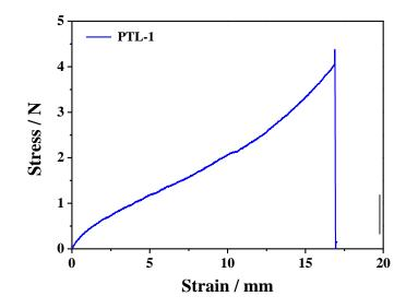
**Figure 3.6.** Tensile tests (reported as Stress/Strain curve) carried out on sample PTL-1 according to ASTM Standard D638, using a Sintech 10/D instrument equipped with an electromechanical extensometer (clip gauge).
