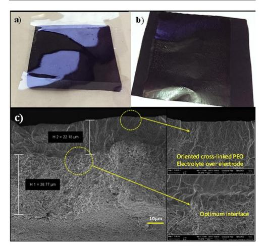
**Figure 3.13** (a) Photograph of bare TiO<sub>2</sub> based electrode and electrolyte before UV curing. (b) Freshly prepared self-supporting multiphase electrode/electrolyte composite obtained by direct hot-pressing and in situ photopolymerisation of the polymer electrolyte over the TiO<sub>2</sub>-electrode film supported over copper foil. (c) Cross-sectional FESEM images showing the optimum interface achieved after UV curing.
