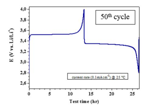
**Figure 3.16** Charge/discharge curve of a lithium test cell assembled with a configuration of Li/PTL-1/LiFePO<sub>4</sub>. The test was performed at 25 °C at current densities of 0.1 mA cm<sup>-2</sup>.
