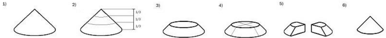
Figure 7: Schematic representation of coning-quartering sampling method
