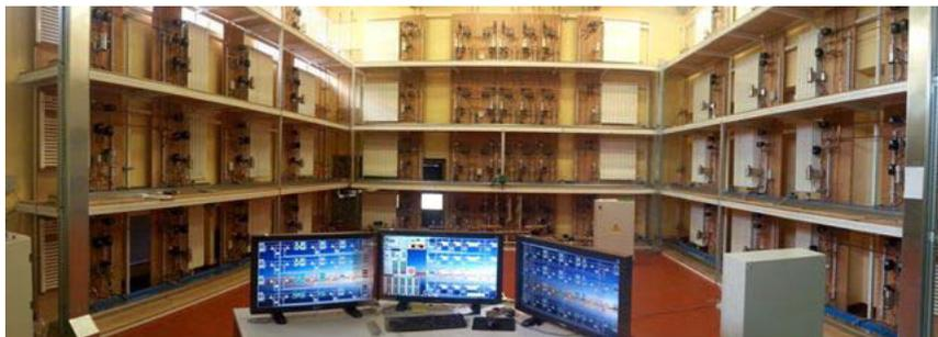
Fig. 1. Overview of the thermo-hydraulic circuit of the central heating system simulator
