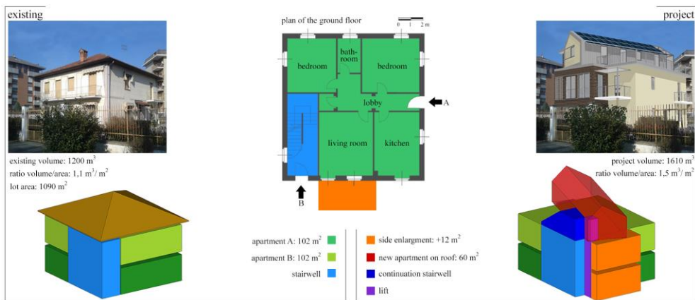
Fig. 2. The residential building used as case-study: existing and project schemes (the second floor having the same layout of ground floor).
