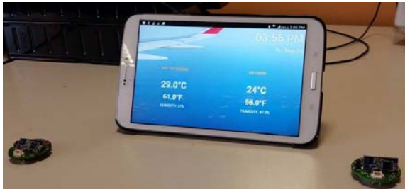
Fig. 6. Main Interface of the BLE-based android application for acquiring environmental data.
