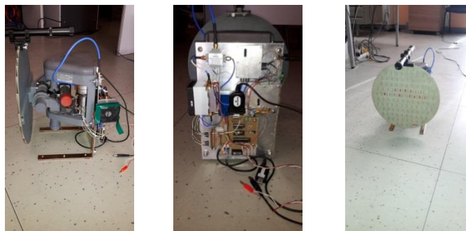
FIG. 2 – The realized prototype of multipurpose low cost FMICW radar.
