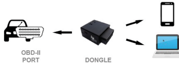
Fig. 9. A dongle can be connected to the OBD-II port to allow brought-in devices to access vehicle data.
