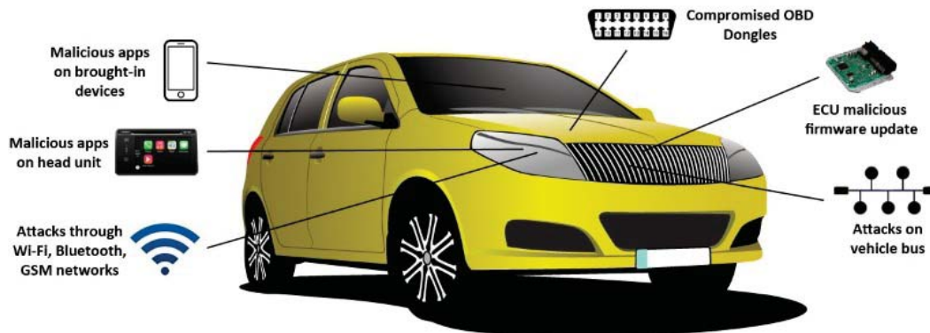
Fig. 11. Some examples of issues for connected car security. (Vector Graphic Source: http://www.WebDesignHot.com )
