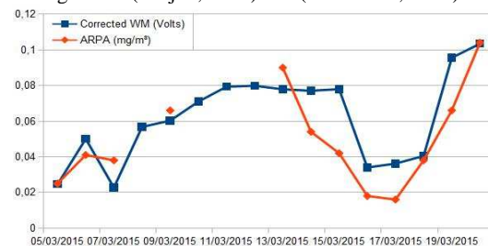
Figure 2. Calibration of the dust sensor.
