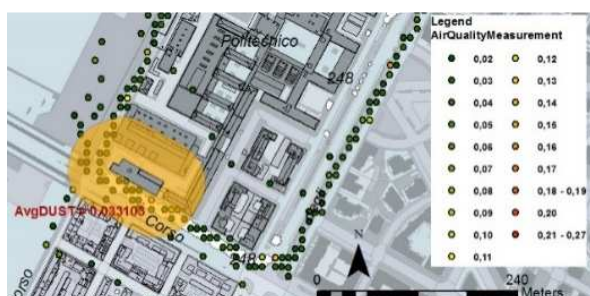
Figure 6: GIS layout showing an example of possible spatial analysis of dynamic data in the area of the Politecnico in Turin: the average of the values measured in a 50 m buffer of a buildings can be calculated and associated to the selected building.
