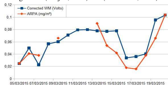
Figure 2. Calibration of the dust sensor.
