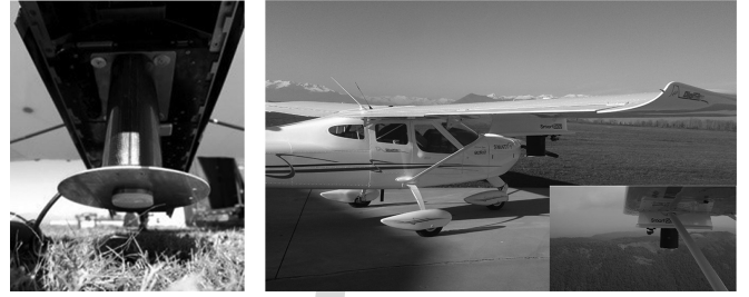
Fig. 3. GNSS-R prototype mounted on digisky P92 aircraft.
