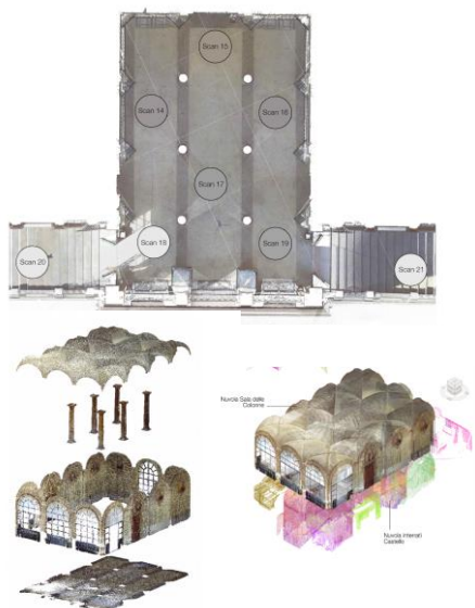
Figure 9. Point cloud segmentation before scan to BIM modelling in Revit
