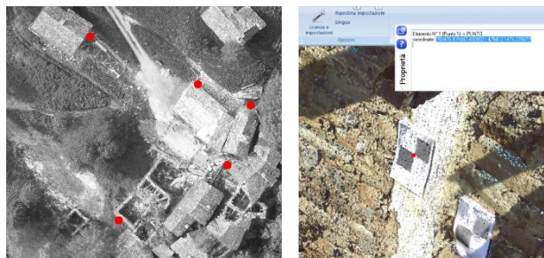
Figure 15. Marked CPs and measured coordinates on the target in registered cloud for a following comparison with TS measured coordinates (Table 5).
