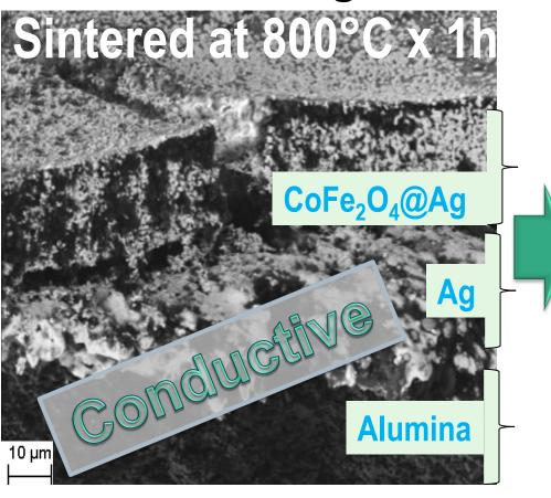
Ag-coated alumina was used to produce CoFe<sub>2</sub>O<sub>4</sub> layer embedded in silver
