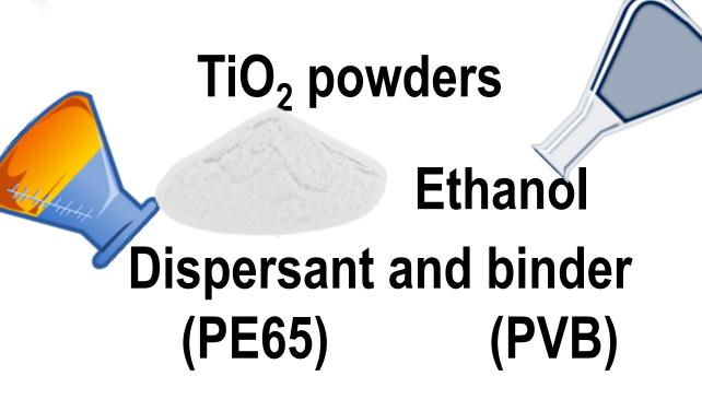
TiO<sub>2</sub> (Degussa P25) **Particles Stoichiometry:**  $0.88 \text{ g/cm}^{-3}$ **Suspension Density:** Solid Loading, wt%: 11.4 Particle Size (DLS): 200 nm
