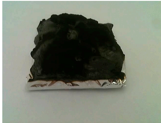
Figure 8. Residue of H/E-15APP after cone calorimetry tests.
