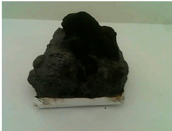
Figure 9. Residue of HT/E-15APP after cone calorimetry tests.
