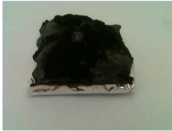
Figure 8. Residue of H/E-15APP after cone calorimetry tests.
