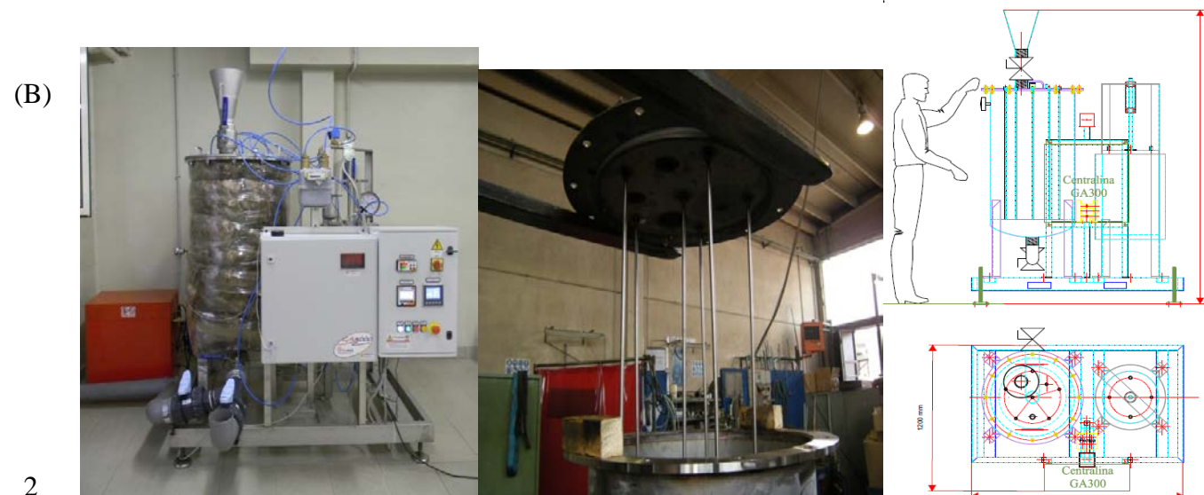
3 Figure 1. Experimental apparatus employed for (A) semi-pilot scale tests and (B) pilot scale tests
