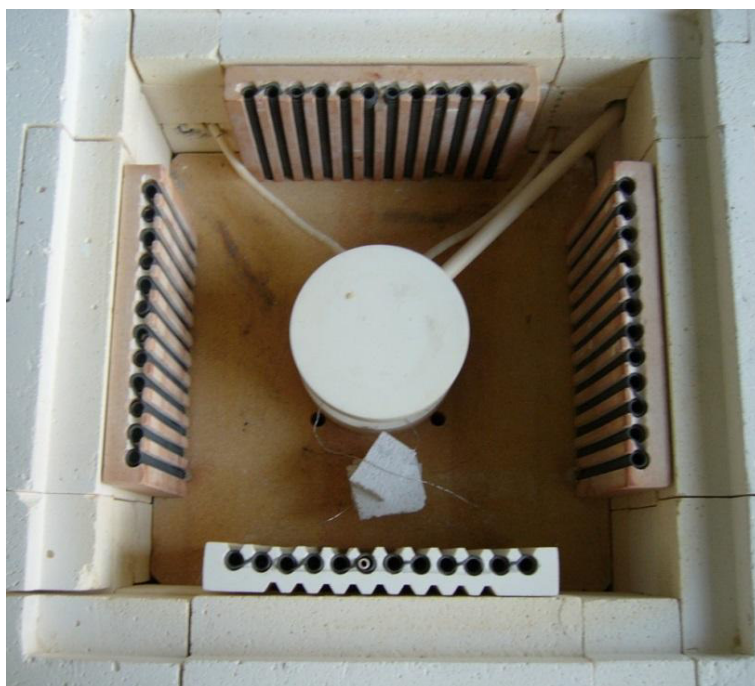
Figure 4.3 – Test-fixture assembled in the test chamber.
