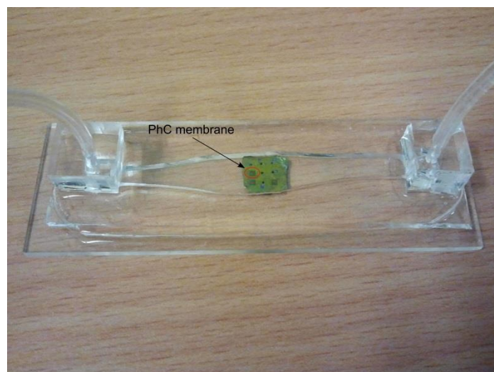
Figure 4.10: Microfluidic system used to test the PhC membrane. The channel has been made in polydimethylsiloxane (PDMS) and placed on a microscope glass slice. Then, it has been covered with a transparent plastic sheet where the inlet and outlet have been obtained. The pipes have been connected to the system by means of two small pieces of PDMS fixed on the plastic sheet using epoxy glue.
