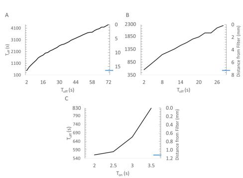
Figure 2.12: Example of operational graph. This graph was obtained for particle diameter equal to 10  $\mu$ m and flow rate 30 mL/min. (A) Graph for an initial particle cloud volume equal to 10 mL, (B) 25 mL, and (C) 40 mL. Blue ticks on the right vertical axis represent the initial distance of the particle cloud, which varies according to the initial cloud volume variations.
