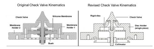
Figure 2.17: Comparison between the original and revised kinematic mechanism of the check valve system visualizing a section of the check valve system both in open position. The number of elements composing the assembly of the revised check valve assembly was consistently reduced.
