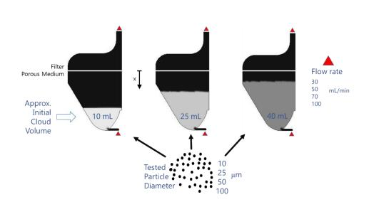
Figure 2.11: Explicative representation of the combination of parameters varied in the multiphysics simulations. x coordinate origin is positioned on the filter to calculate the cloud distance from the filter.
