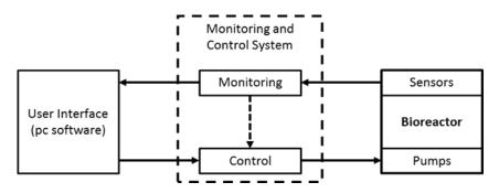
Figure 2.24: Concept chart of the control and monitoring system. Monitoring unit gets the signals from the sensors. These signals (after processing) are showed through the user interface. The user, through the interface, can directly act on control unit to set the pump flow rates in order to adjust pH or DO signals overtime. The dashed arrow represents the future aim to perform an automated control based on monitoring feedback signals.
