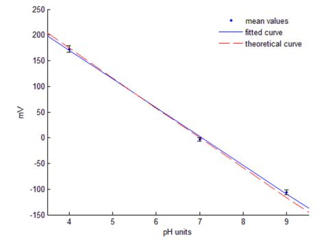
Figure AII.7: Calibration curve obtained after the characterization process.
