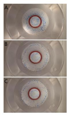
Figure 4.2: Representation of the Cytodex 1 microcarriers: low flow rate are not capable of generating particle suspension (A, 20 mL/min). With increasing the imposed flow rate particles are suspended and homogeneously distributed within the culture chamber (B, 30 mL/min; C, 50 mL/min).
