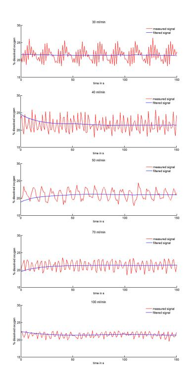
Figure 2.30: DO measurement (red) and filtered signals varying imposed flow rate values.
