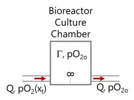
Figure AI.3: Schematic of the bioreactor chamber compartment. The amount of dissolved oxygen within the medium is homogenously consumed with a consumption kinetics  $\Gamma$ .
