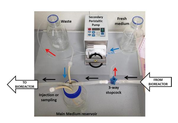
Figure 2.23: Preliminary setup of the continuous perfusion feeding circuit. Red arrows indicate the flow towards the waste bottle. Blue arrows indicate the flow of the fresh medium towards the main reservoir. Horizontal black arrows indicate the flow direction in the closed-loop perfusion loop.
