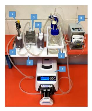
Figure 2.28: Final bioreactor platform configuration. 1, Culture chamber. 2, Downstream sensing flow chamber. 3, Upstream sensing flow chamber. 4, pH and DO sensors. 5, Support. 6, Reservoirs. 7, closed loop recircilation pump. 8, continuous perfusion feeding secondary pump.
