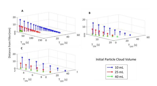
Figure 2.14: Operational graph in form of stem plots for suspended particles of 100  $\mu m$ , varying the flow rate from (A) 50 mL/min, (B) 70 mL/min, and (C) 100 mL/min.
