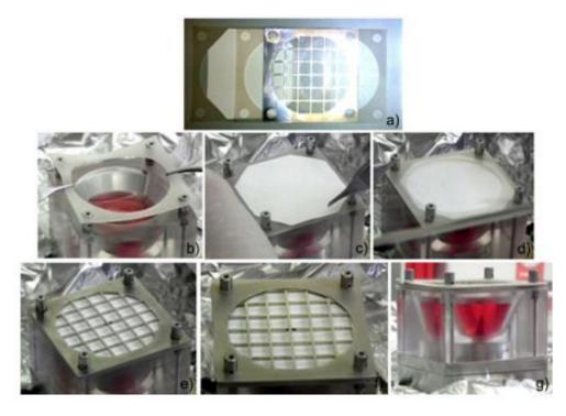
Figure 2.3: Bioreactor filter setup. a) Filter Components, b) insertion of the first silicone washer, c) insertion and positioning of the PVDF filter, d) insertion of the second silicone washer, e) insertion of the AISI 316L stainless steel grate, f) insertion of the third silicone washer, g) completed filter setup.
