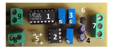
Figure AII.5: realized amplification/polarization circuit.
