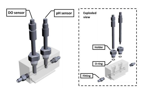
Figure 2.26: Sensing flow chamber 3D model. Left panel, the assembled flow chamber including sensors. Right panel, the exploded view with all the components (holders, o-tings, fittings, sensors).
