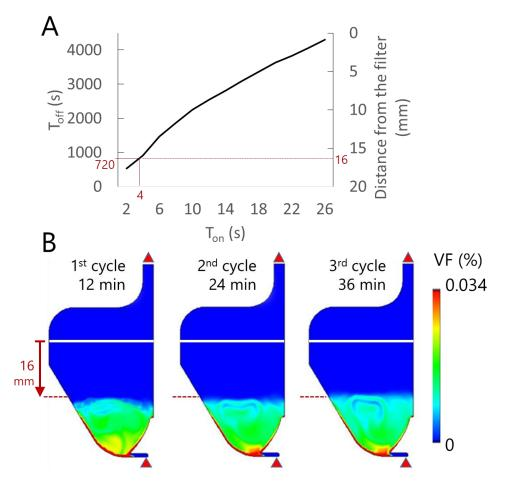
Figure 2.15: Example of application of the pulsed protocol by the application of the operational graphs for suspended particles with diameter of 10  $\mu$ m and flow rate equal to 50 mL/min. (A) Chosen the minimum distance from the filter of the particle cloud (16 mm), the couple  $T_{on} / T_{off}$  is determined ( $T_{on} = 4$  s  $T_{off}$ , =720 s or 12 mins). (B) VF distribution describing the particle cloud at the end of every simulated pulsed cycle.
