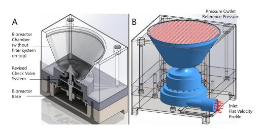
Figure 2.20: Final implementation of the revised check valve system within the bioreactor 3D model (A). This implementation was used for the definition of the computational domain (B) used for the in silico computational optimization of the design.
