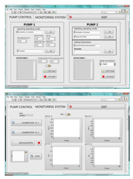
Figure AII.10: Screenshot of the realized control unit software. (top) View of the monitoring system window, and (bottom) the control system window with its dialog blocks.
