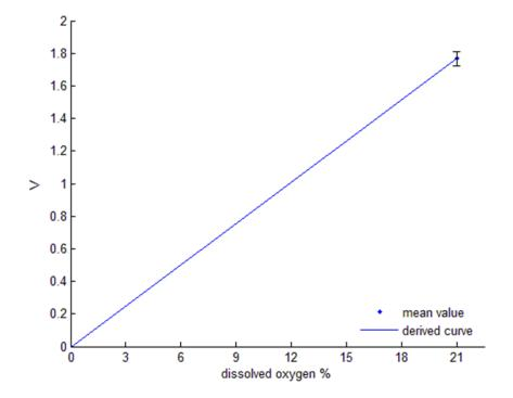
Figure AII.8: Calibration curve obtained after the DO sensor characterization.
