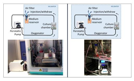
Figure 2.5: Bioreactor setup within the incubator in two possible configurations. Schematic drawings (top) and pictures of the real working system (bottom). The peristaltic pump can be put outside the culture incubator in case of high humidity (left panel) or cab be positioned inside the incubator in absence of humidity (right panel).
