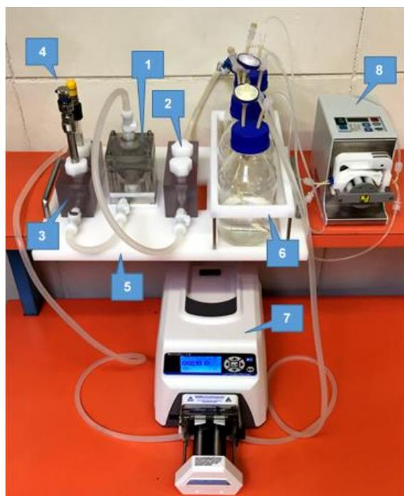
Figure 2.28: Final bioreactor platform configuration. 1, Culture chamber. 2, Downstream sensing flow chamber. 3, Upstream sensing flow chamber. 4, pH and DO sensors. 5, Support. 6, Reservoirs. 7, closed loop recirculation pump. 8, continuous perfusion feeding secondary pump.
