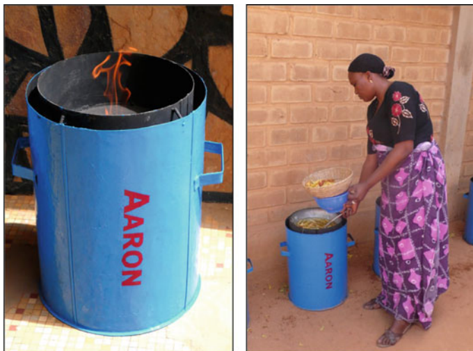
Fig. 15.7 The gasification stove developed
