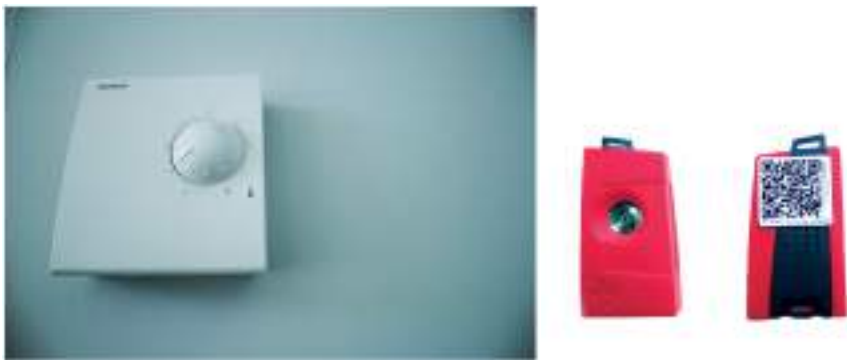
Fig. 32 Thermostat for temperature regulation (left) and wearable smart sensor (right) for temperature and humidity measurements used in the Comfrotsense Project
