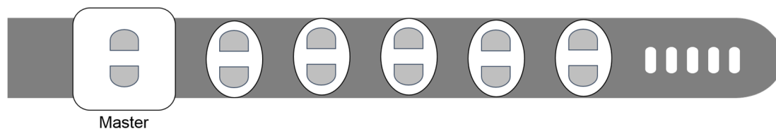
Fig. 122. Concept of sEMG armband. The armband is composed by six dry-electrodes and one of them is the master, which provide also the signal conditioning and the appropriate gains.
