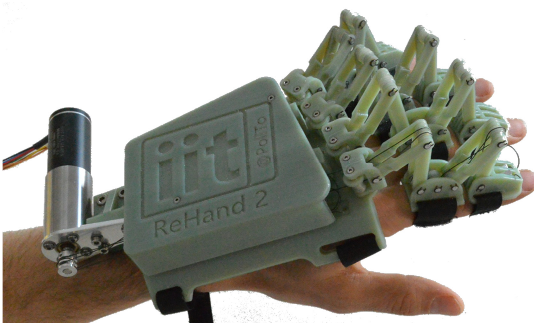
Fig. 72. Proof of concept of a bidirectional tendon-driven underactuated hand exoskeleton, namely ReHand2
