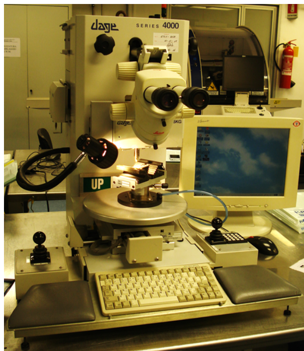
FIGURE A.2: Nordson DAGE Shear tester - utilized instrument.
