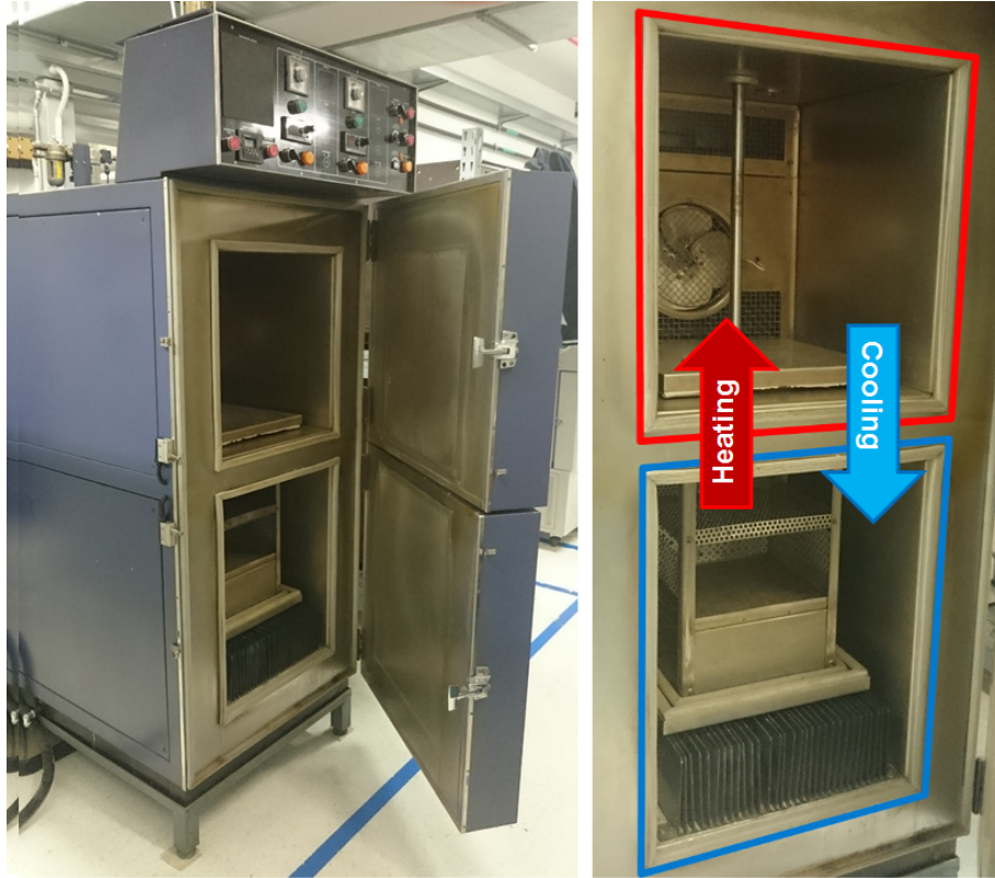
FIGURE 3.10: Test chamber utilized for Temperature Cycling Test.
