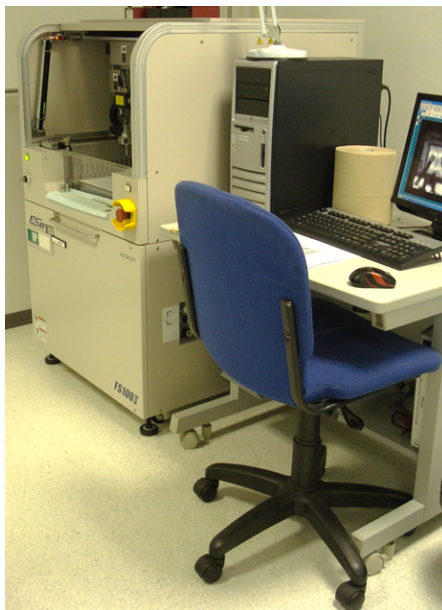
FIGURE B.5: Scanning Acoustic Microscopy utilized.
