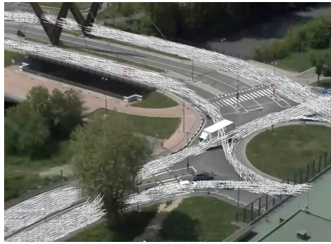
Figure 6. Learning the flow model: the directions stored in the grid cells are super-imposed on a camera image.
