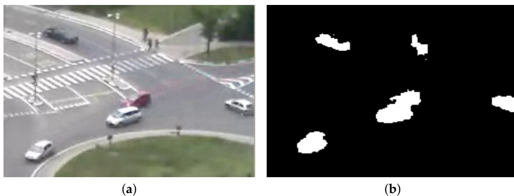
Figure 4. Object detection phase: (a) initial image; and (b) detected objects. Notice the top-right segmented objects, corresponding to a pedestrian group, which will be filtered-out in the following layer.
