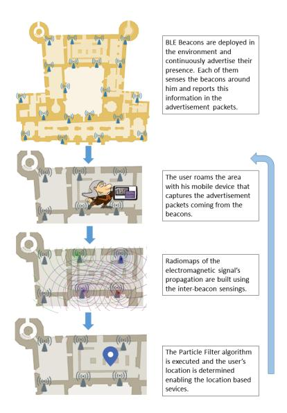
Figure 5.3: Schema of the proposed solution.
