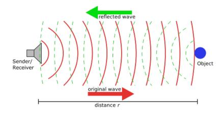
Figure 4.7: Sonar principle
