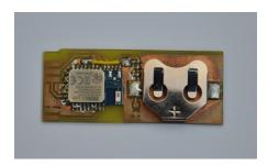
Figure 5.5: First version of the network nodes.
