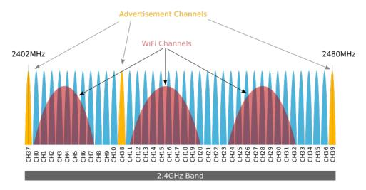
Figure 5.4: Bluetooth Low Energy channels.
