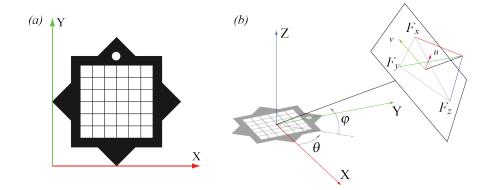
Figure 3.1: The marker used in the Step by Step applications (a) and the relative position of camera and marker (b).
