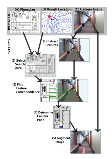
Figure 4.9: Hile's and Borriello's system diagram for calculating camera pose and overlaying information on an image from a camera phone.
