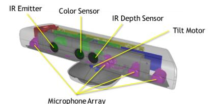
Figure 4.12: The Kinect sensor components. Picture from https://msdn.microsoft.com/en-us/library/jj131033.aspx.
