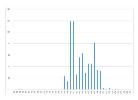
Figure 5.7: RSSI values distribution as sensed by the mobile devices placed at one meter from both anchors.
