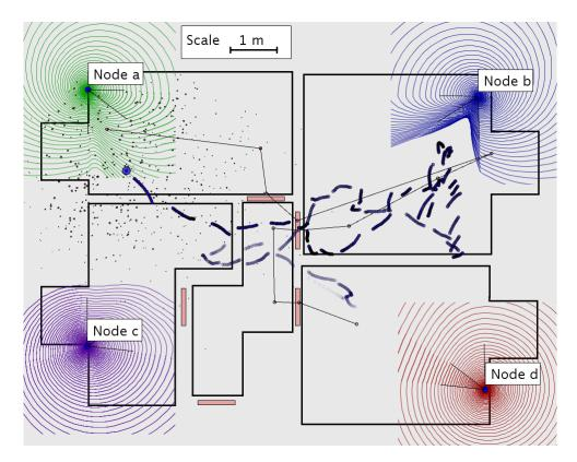
Figure 5.18: Result of the execution of the positioning algorithm. The radio-maps are scaled down for illustration purposes.
