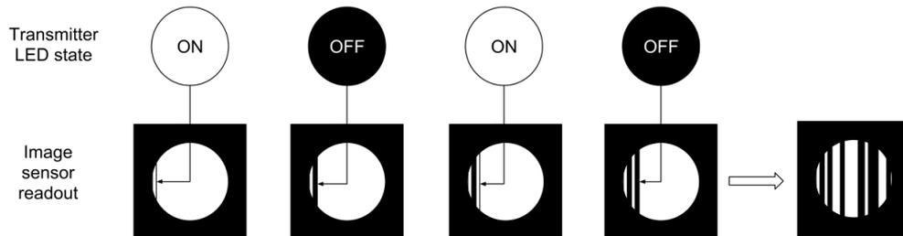
Figure 4.10: VLC data frame sample. Image from [108].
