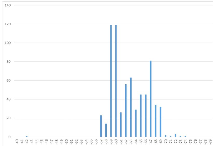
Figure 5.7: RSSI values distribution as sensed by the mobile devices placed at one meter from both anchors.
