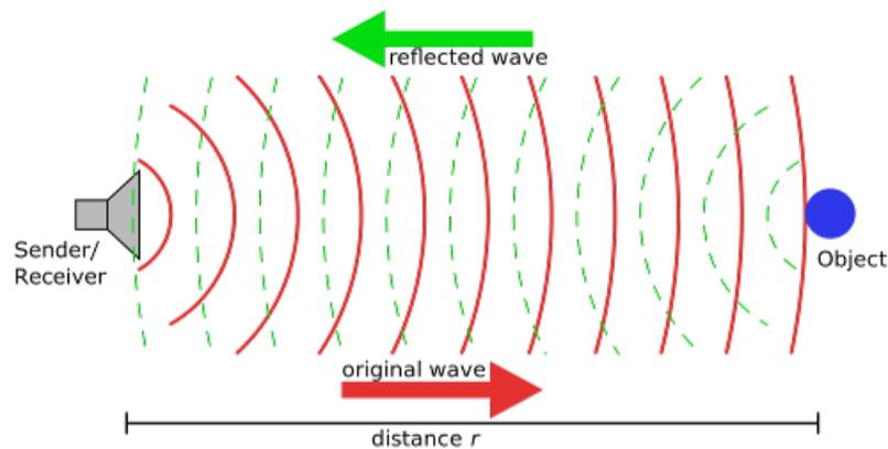
Figure 4.7: Sonar principle
