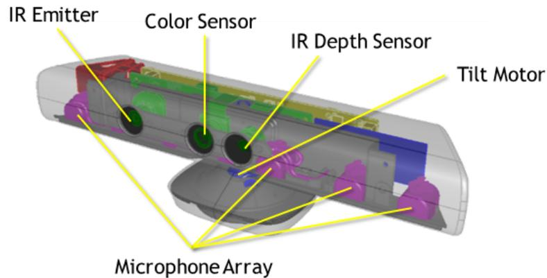
Figure 4.12: The Kinect sensor components. Picture from <https://msdn.microsoft.com/en-us/library/jj131033.aspx>.
