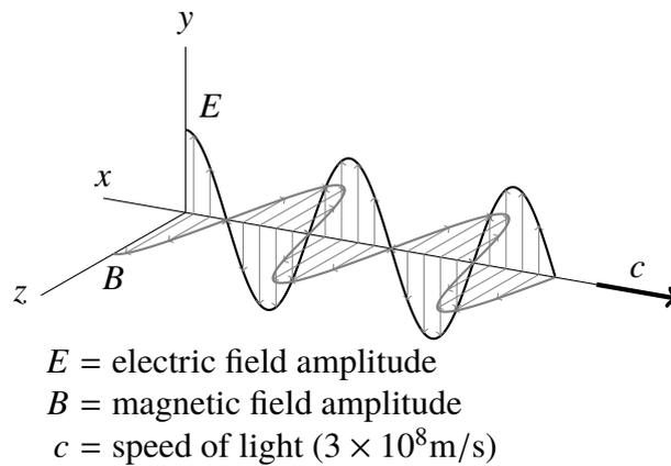
Figure 4.21: Electromagnetic wave.
