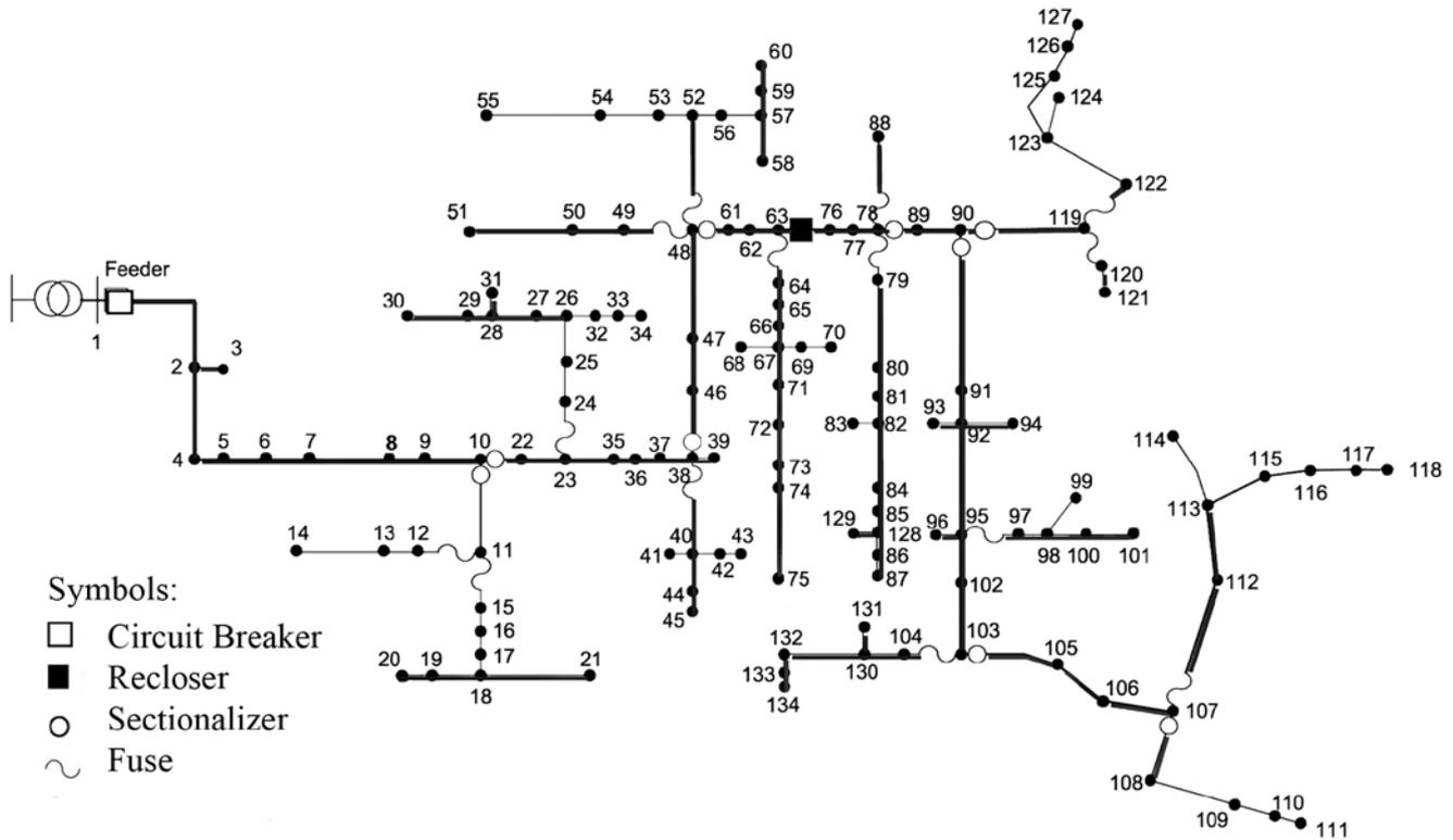
Fig. 1. Single line diagram of 134 node distribution feeder [13]
