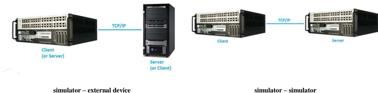
Figure 12 TCP/IP and UDP/IP Configurations for RTs (Opal or RTDS)
