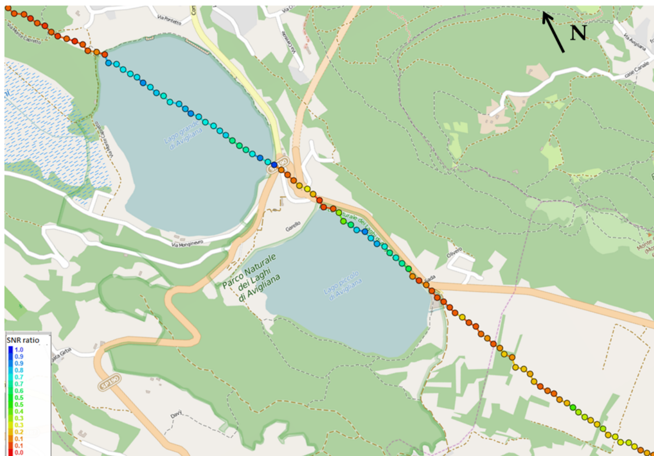
Figure 10. Specular points of PRN 30 over the Avigliana lakes. The color is proportional to the SNR ratio between the left-hand circular polarized (LHCP) reflection and the direct GPS signal.
